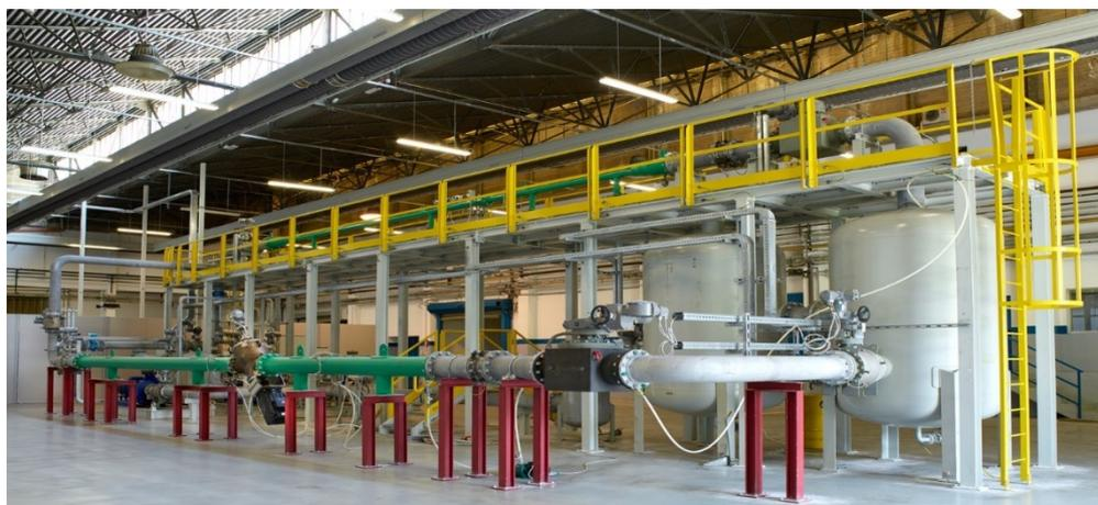
*LOCPOWER energy harvesting valve during a flow test in our Valpres facility*
